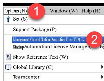
Figure 5-9-2 Installing GSD files
