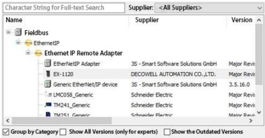
Figure 5-7-17 Adding the EX-1120 adapter
