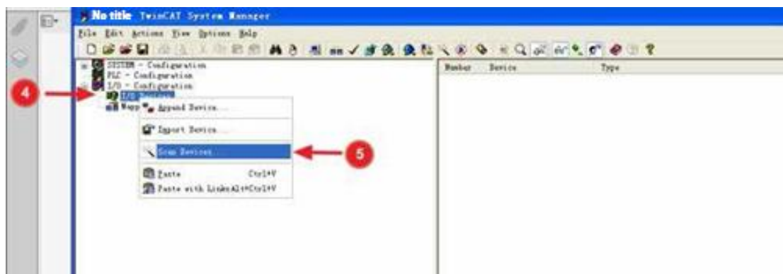
Figure 5-1-4 Selecting Scan Devices
