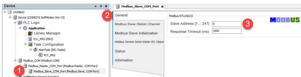
Figure 5-6-18 Configuring the master protocol and related timeout parameters
