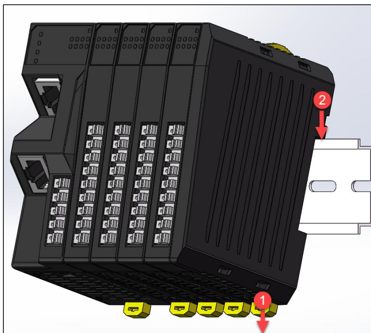
Figure 3-2 Installing an entire module group
