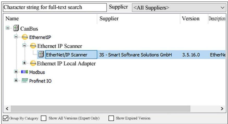
Figure 5-8-15 Adding the EthernetIP scanner
